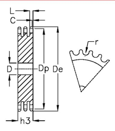
C = 2 D = 25 De = 318.4 Dp = 309.45 For chain size =  $3/4 \times 7/16$ For chain type = 12 B-3 h3 = 49.8 L = 10.8 Number of teeth = 51r = 12.07
